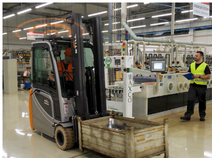
warning zone - forklift autonomously decelerates, personal tag vibrates
